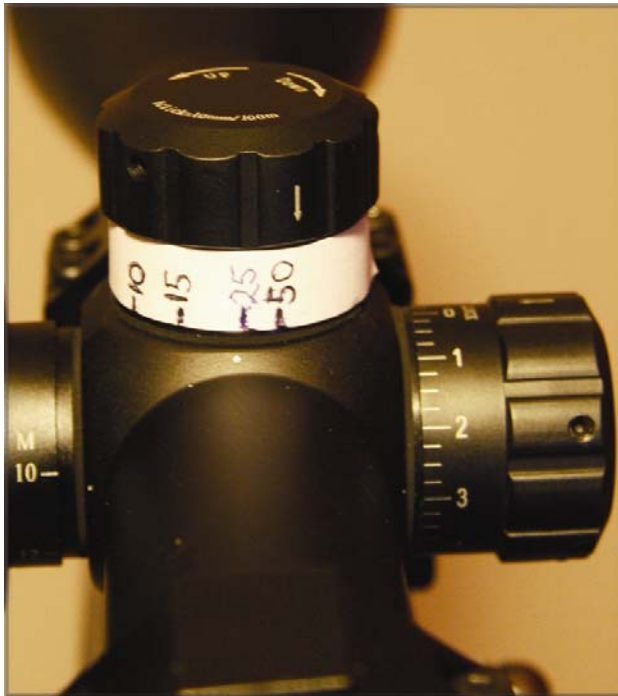
Locking turrets are great and marking the dial with tape allows perfect zero at all distances
